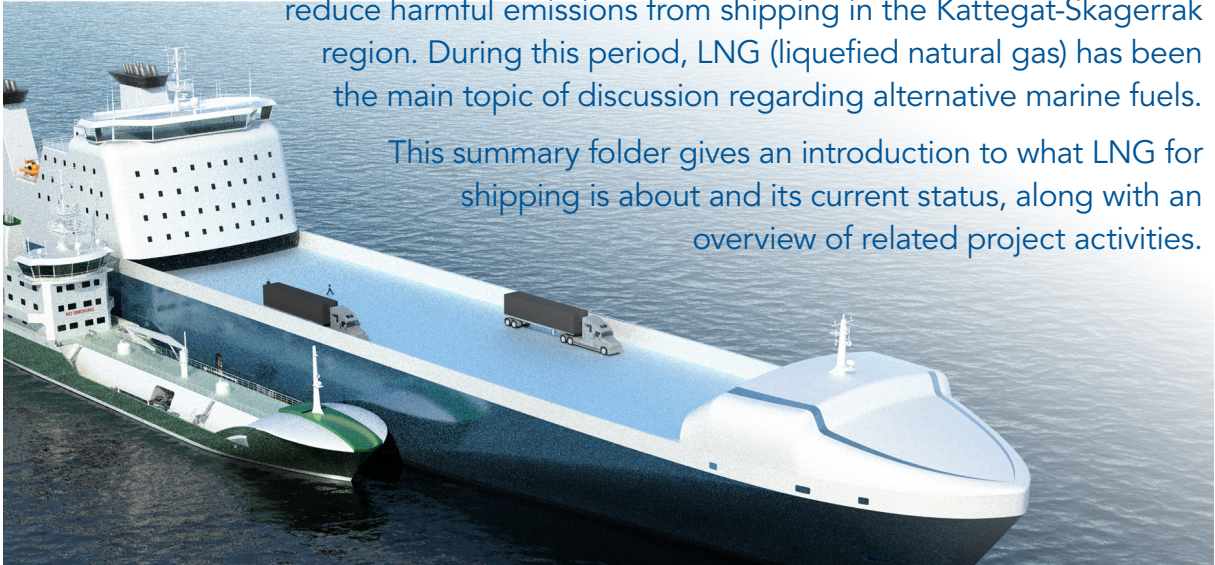
Illustration of LNG ship-to-ship bunkering. Picture by FKAB Marine Design.
